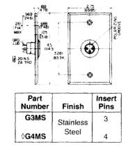
Wall plate with one B3M or B4M male receptacle mounted (in "D"-shaped hole to prevent turning) on standard single electrical outlet box. Cover mounting screws included.
