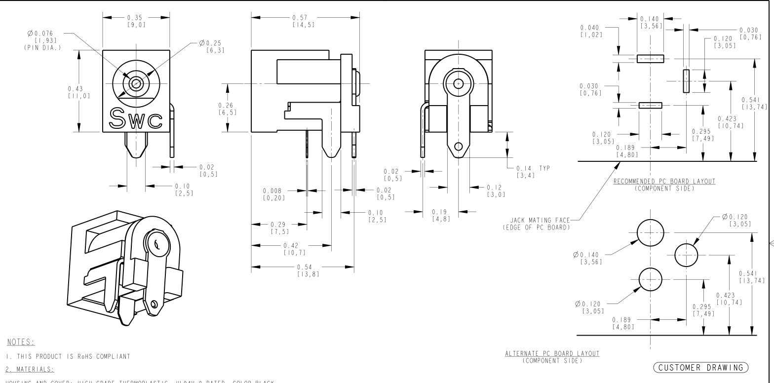
HOUSING AND COVER: HIGH GRADE THERMOPLASTIC, UL94V-0 RATED, COLOR BLACK. CENTER PIN: BRASS, NICKEL PLATED PER QQ-N-290, CLASS I. PIN AND SHUNT TERMINALS: BRASS, SILVER PLATED PER QQ-S-365. SLEEVE SPRING: SPRING COPPER ALLOY, SILVER PLATED PER QQ-S-365.
