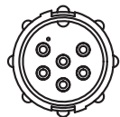
6 POSITION #20 PIN & SOCKET CONTACT
