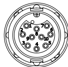
10 POSITION #22 PIN & SOCKET CONTACT
