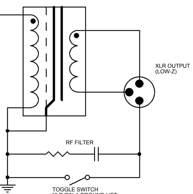
FULLY SHIELDED IMPEDANCE MATCHING TRANSFORMER
