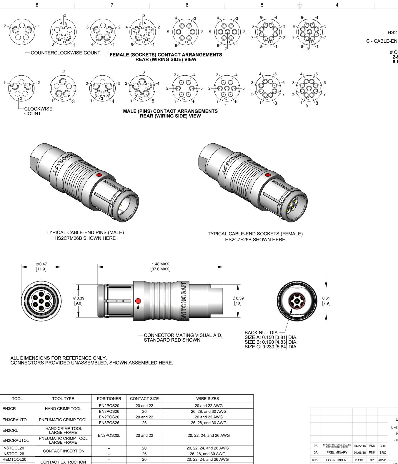
HS2 C KIT PACKAGING OPTION: **K** - ONE UNIT / BAG HS2 SERIES C - CABLE-END CONNECTOR CLAMP SET PER CABLE O.D. RANGE: **A** - 0.110 - 0.140 [2.8 - 3.6] **B** - 0.140 - 0.180 [3.6 - 4.6] **C** - 0.180 - 0.216 [4.6 - 5.5] # OF CONTACTS:
