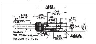
No. 280 typical – shown with solder lug terminals, cord clamp and shielded handle.
