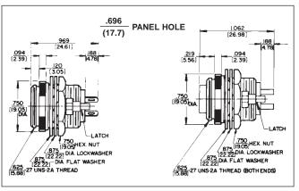
Front of panel mount; 2 through 5 pins (male) or 2 through 5 contacts (female). Also 2-, 3- and 4-contact insert with 3 shunted (N.C.) contacts. Mounting locknut (Part Number SL01), lockwasher (Part Number SL02), and flat washer (Part Number SL03) supplied.
