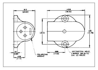
3-pin plug shorts out unused hi-Z microphone inputs or other sensitive circuits (shorting jumper installed between pins 2 and 3). 6" (152.4 mm) chain fastened to end pin to prevent plug loss. Switchcraft can install special wiring for a nominal extra charge.
