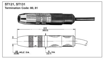
**ST121:** Straight Extension Jax<sup>®</sup> jack is a shielded 2-conductor jack with .50" (12.7 mm) outside diameter. Cable clamp connects shield or second conductor to cable. Mates with .25" (6.35 mm) diameter Switchcraft 2-conductor plugs.
