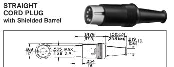
**Type 15GM7M – typical:** Male cord plug with shielded barrel and insulated snaplock plastic body. Two piece metal barrel surrounds pin insert to form an electrical shield. The entire insert assembly is held together by snapping the insulated plastic shell over the assembly. The barrel's special metal tab locks the shell in place. Standard color of plastic shell is gray. All-purpose cable clamp.
