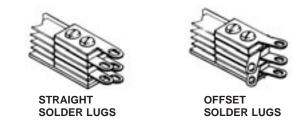
**WIRE-WRAPPING TERMINALS** – Wire-wrapping eliminates the need for soldering. Each terminal accepts up to three wrapped wires (22 or 24 gauge, 5 wraps each), applied with standard wire-wrapping tools. Terminal base has standoff shoulder which prevents first wrapped wire from accidentally sliding down and shorting against another terminal or adjacent spring. Terminal tips are radiused to facilitate positioning of wire-wrapping tool over terminals. See page 80 for wire-wrapping data.
