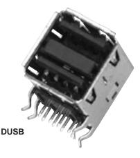
Switchcraft introduces single and dual USB connectors. The USB connectors are fast becoming the industry standard for plug and play connectivity between PCs and their peripherals. The DUSB and USB connectors are RAPC mounted, with kinked terminals for snap-in placement to the PC board. Both meet all Universal Serial Bus standards.
