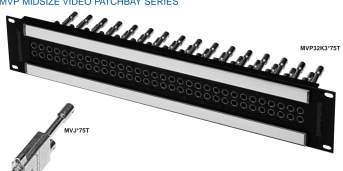
The MVP Series video patchbays offer outstanding performance and high density. Patchbays consist of 32 jacks in either 1RU or 2RU heights, jacks come either terminated or non-terminated. These jacks are rated from DC to 3 GHz, and are rated at 30,000 lifecycles.
