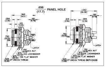
Front of panel mount; 2 through 5 pins (male) or 2 through 5 contacts (female). Also 2-, 3- and 4-contact insert with 3 shunted (N.C.) contacts. Mounting locknut (Part Number SL01), lockwasher (Part Number SL02), and flat washer (Part Number SL03) supplied.
