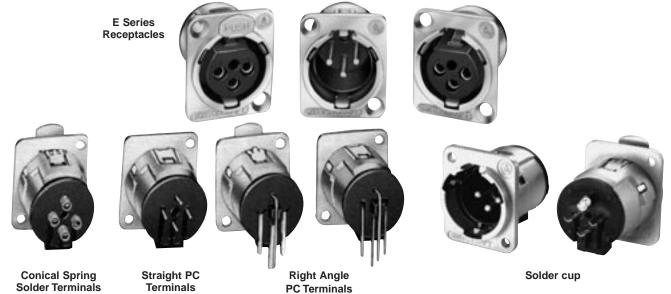
E Series Q-G $^{\circ}$  Receptacles are available with quick release inserts. Quick insert release is accomplished by turning screw lock from front of insert. Insert can then be removed from the rear. For PC board applications, insert can be removed/assembled to the housing while soldered to the PC board.
