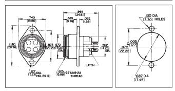
Flange mounted; 2 through 5 pins (male) or 2 through 5 contacts (female). Also 2-, 3- and 4-contact inserts with 2 shunted (N.C.) contacts.
