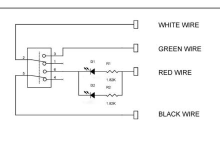
SCHEMATIC CIRCUIT 1A WITH LEDs
