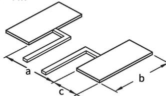
Not following the recommended land pattern design can seriously affect the temperature coefficient measurement results and current sensing accuracy!
