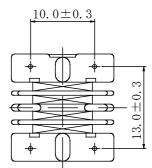
\* Dimension does not include solder used on coil.
