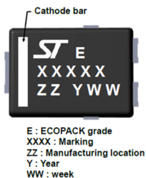
Figure 10. PSMC (TO-277A) marking
