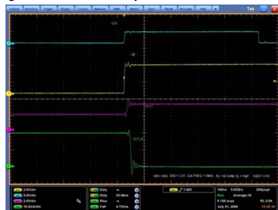
Figure 17: Turn OFF output current characteristics (2)
