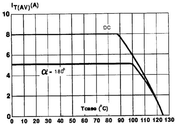
Fig.6 : Average on-state current versus case temperature (TYN).
