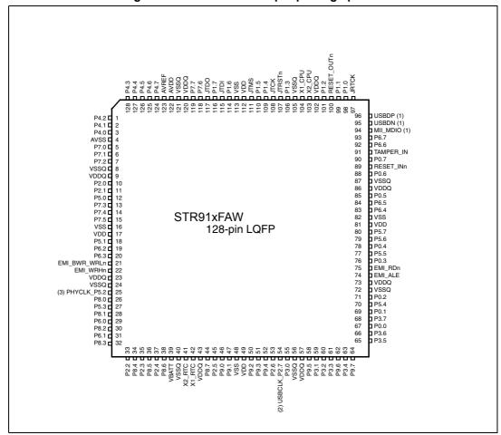
Figure 8. STR91xFAW 128-pin package pinout
