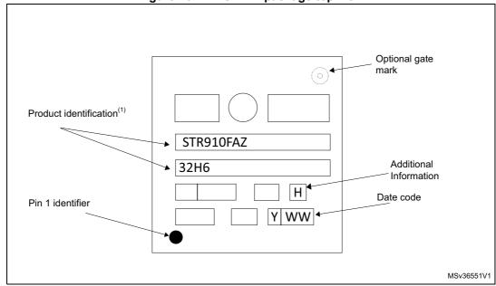
Figure 46. LFBGA144 package top view
