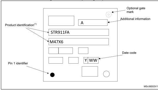
Figure 42. LQFP80 package top view
