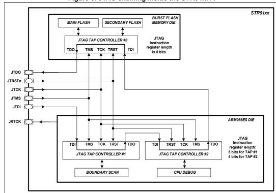
Figure 3. JTAG chaining inside the STR91xFA
