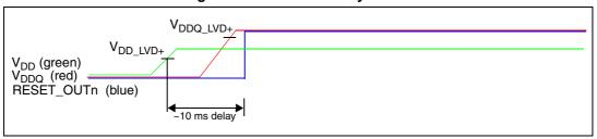
Case 3: When  $V_{DD}$  reaches the  $V_{DD\_LVD+}$  threshold after the  $V_{DDQ}$  rising edge, RESET\_OUTn will be released at the end of a ~10 ms delay. See *Figure 14*
