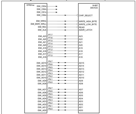
Figure 4. EMI 16-bit multiplexed connection example
