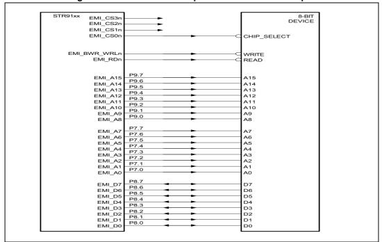
Figure 6. EMI 8-bit non-multiplexed connection example
