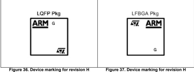
Figure 36. Device marking for revision H LQFP80 and LQFP128 packages
