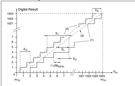
Figure 33. ADC conversion characteristics
