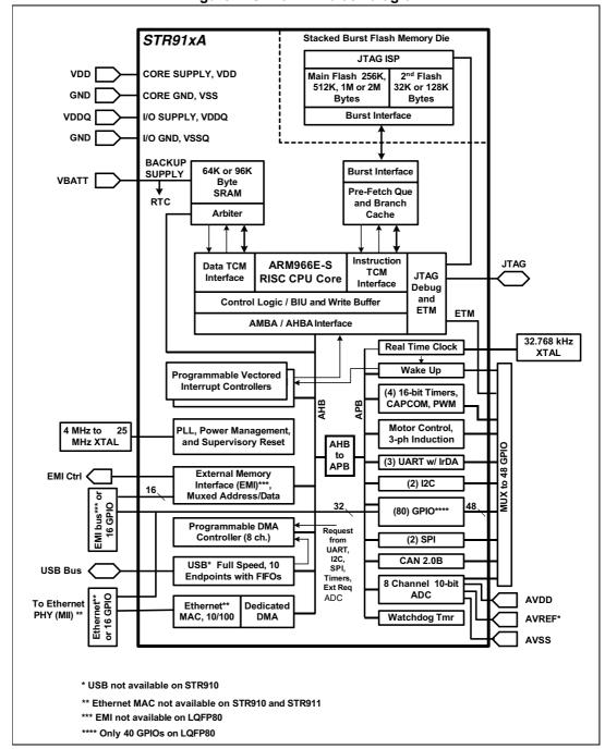
Figure 1. STR91xFA block diagram
