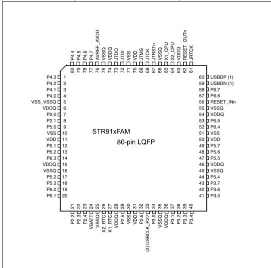
Figure 7. STR91xFAM 80-pin package pinout
