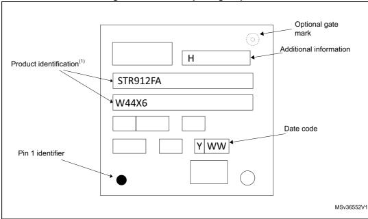
Figure 44. LQFP128 package top view
