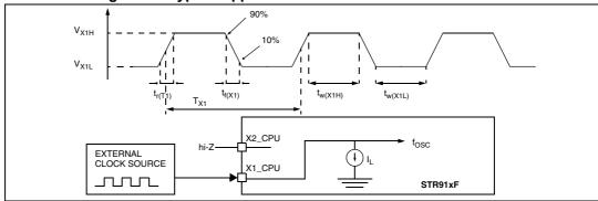
Figure 16. Typical application with an external clock source
