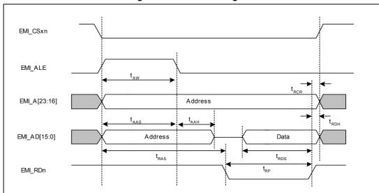
Figure 21. Mux read diagram
