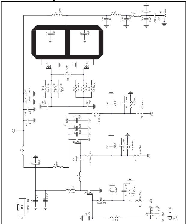
Figure 1. STEVAL-TDR031V1 circuit schematic
