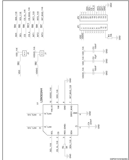
Figure 1: STEVAL-MKI173V1 circuit schematic
