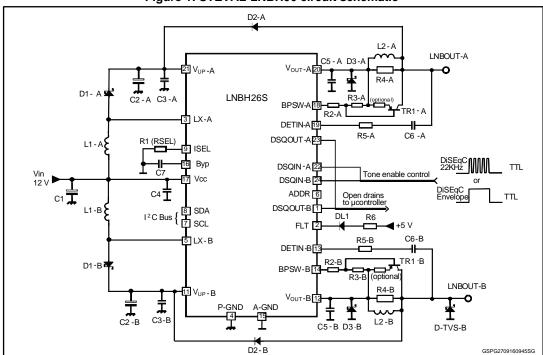
Figure 1: STEVAL-LNBH06 circuit schematic
