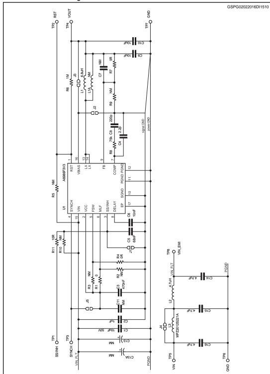
Figure 1: STEVAL-ISA188V1 schematic circuit
