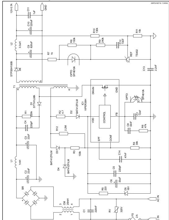
Figure 1: STEVAL-ISA182V1 circuit schematic
