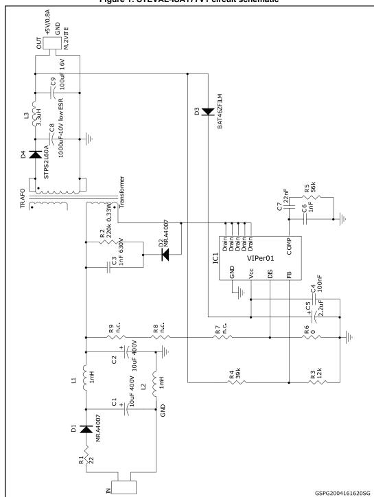
Figure 1: STEVAL-ISA177V1 circuit schematic
