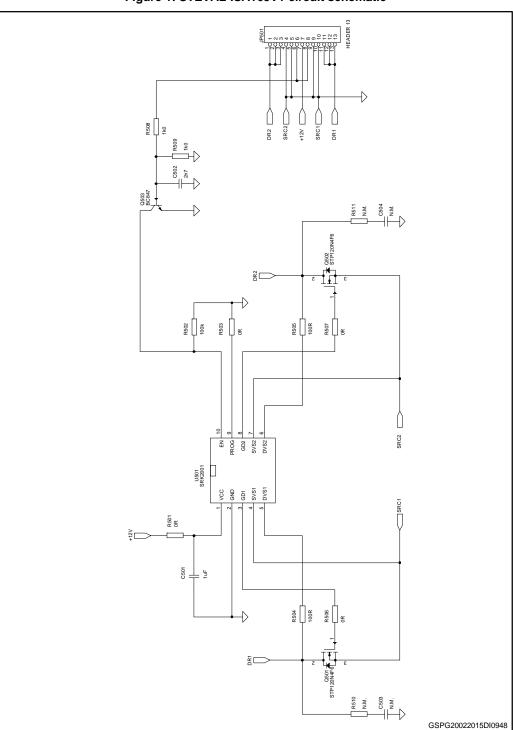
Figure 1: STEVAL-ISA165V1 circuit schematic
