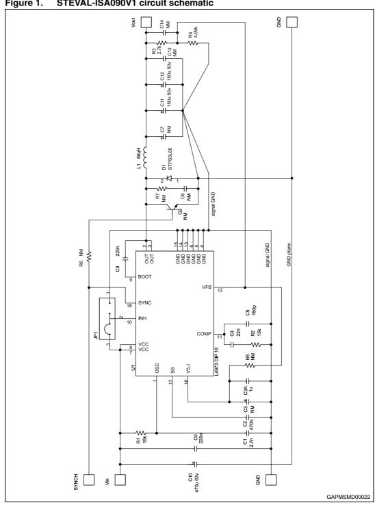
Figure 1. STEVAL-ISA090V1 circuit schematic
