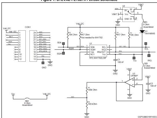
Figure 1: STEVAL-FET001V1 circuit schematic
