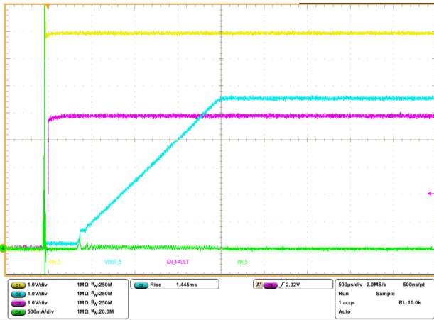
Figure 24. Startup into voltage clamp
