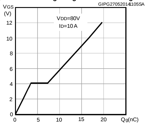
Figure 6: Gate charge vs gate-source voltage
