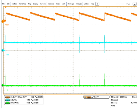
Figure 12. Output ripple, V_{IN} = 3.6\text{ V} , V_{OUT} = 1.8\text{ V} , I_{OUT} = 1\text{ mA}
