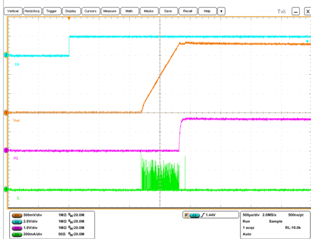
Figure 16. Startup, V_{IN} = 3.6\text{ V} , V_{OUT} = 1.8\text{ V} , no load
