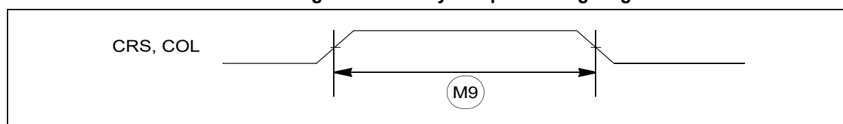
Figure 32. MII async inputs timing diagram
