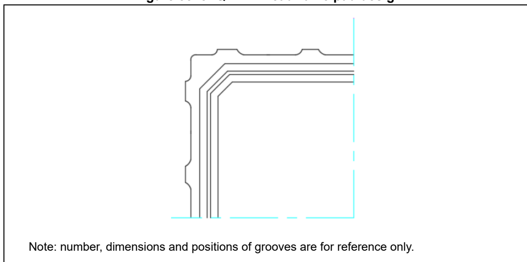
Figure 58. eTQFP144 leadframe pad design
