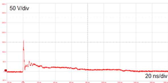
Figure 4. ESD response to ISO 10605 - C = 150 pF, R = 330 \Omega (+8 kV contact discharge)
