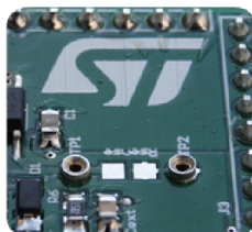
Figure 4. Mounting through-hole sense resistor
