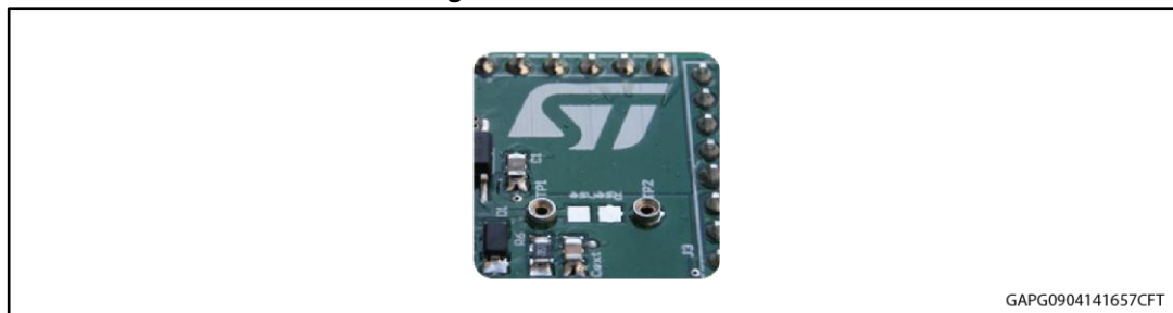
Figure 4: Mounting through-hole sense resistor
