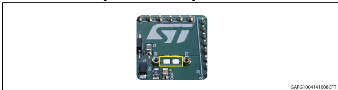
Figure 5: Pads for soldering SMD resistor
