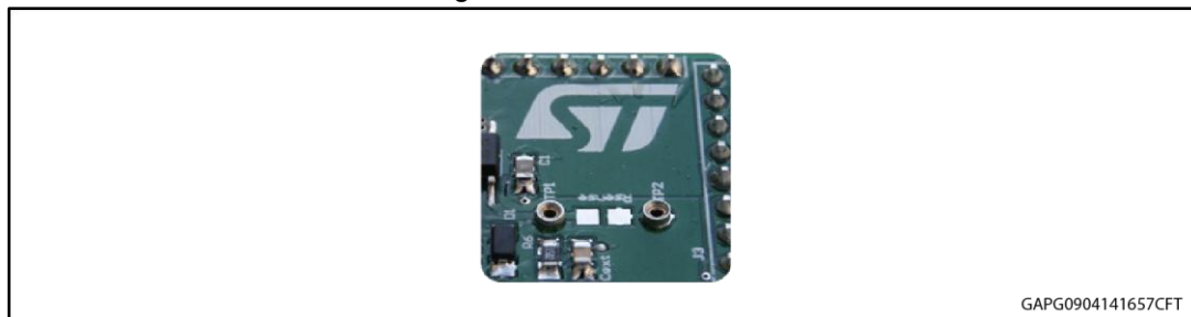
Figure 4: Mounting through-hole sense resistor
