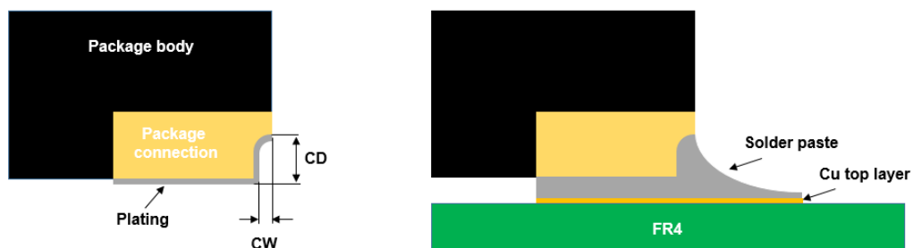
Figure 22. Wettable flank profile
