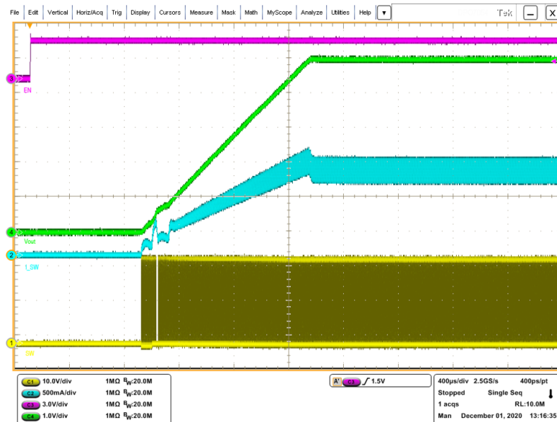
Figure 6. Soft-start phase with I_{OUT} = 1.25\text{ A}
