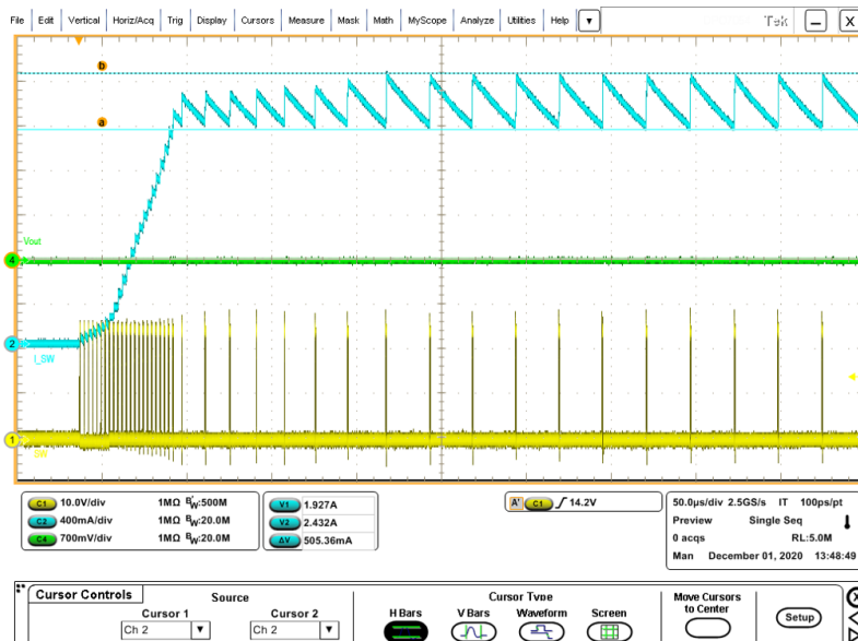
Figure 21. Soft-start procedure with VOUT shorted to GND
