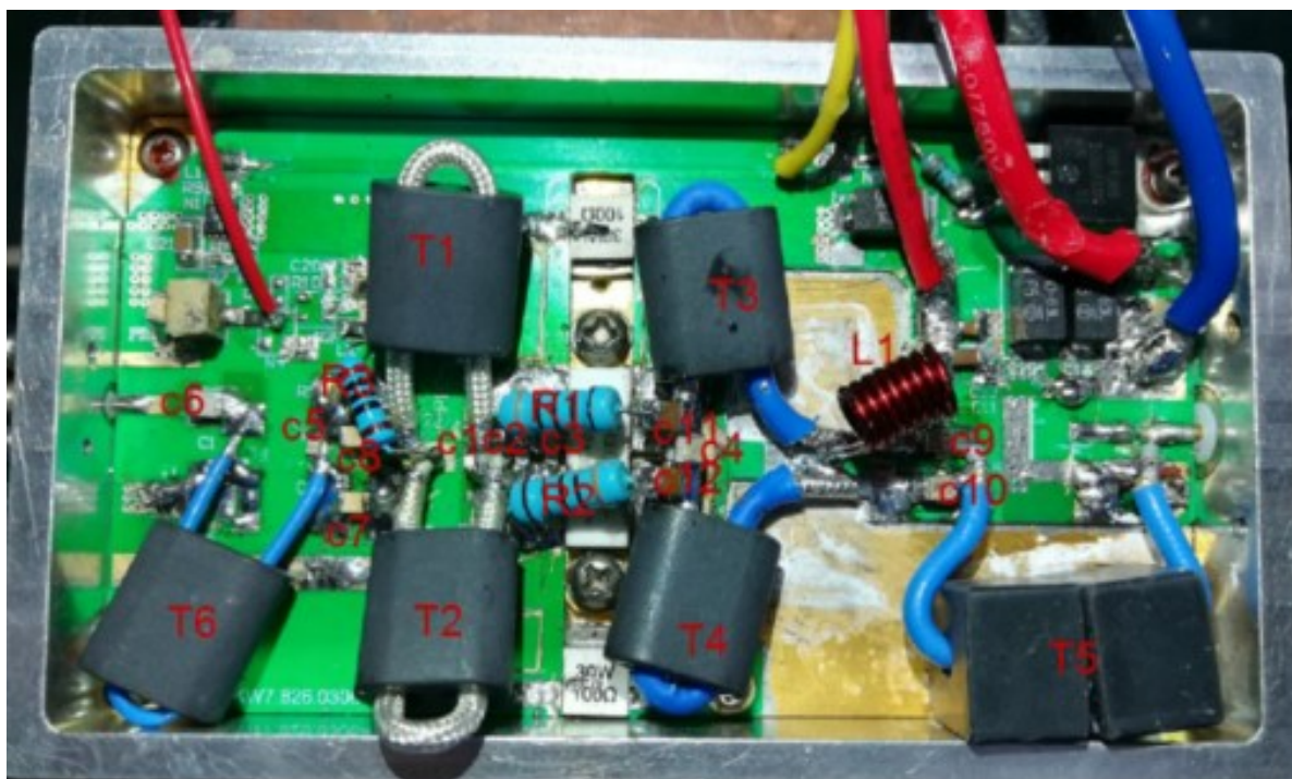
Figure 9. Test circuit photo (broadband)
