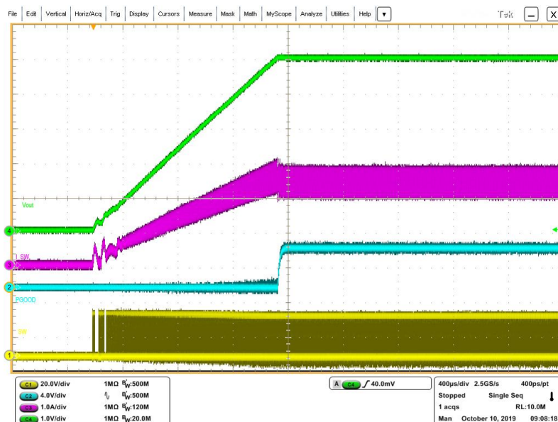
Figure 6. Soft-start phase with I_{OUT} = 2.5\text{ A}
