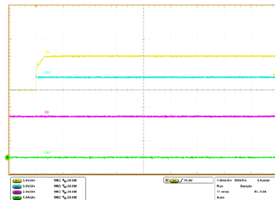
Figure 29. Voltage clamp during operation
