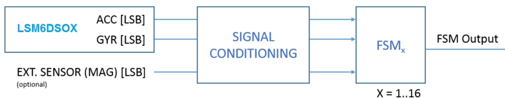
Figure 2. State machine in the LSM6DSOX
