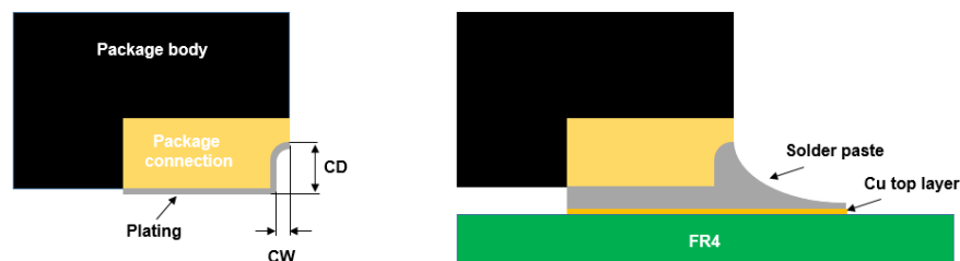
Figure 17. Wettable flank profile
