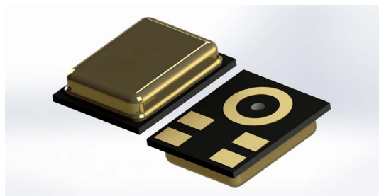
RHLGA metal cap 5-lead 3.5 x 2.65 x 0.98 mm
