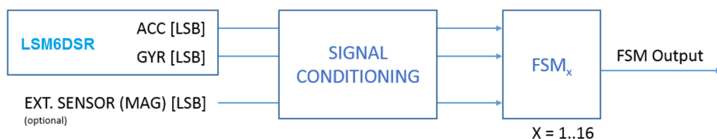
Figure 2. State machine in the LSM6DSR
