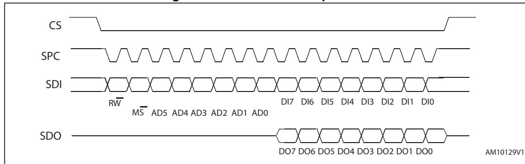
**CS** is the serial port enable and is controlled by the SPI master. It goes low at the start of the transmission and returns high at the end. **SPC** is the serial port clock and is controlled by the SPI master. It is stopped high when **CS** is high (no transmission). **SDI** and **SDO** are respectively the serial port data input and output. These lines are driven at the falling edge of **SPC** and should be captured at the rising edge of **SPC**.
