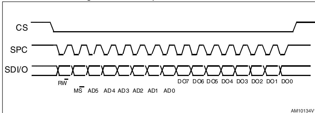
**Note:** Data on CS, SPC, SDI and SDO refer to pins: CS\_A, CS\_G, SCL\_A/G, SDA\_A/G, SDO\_A / SDO\_G.
