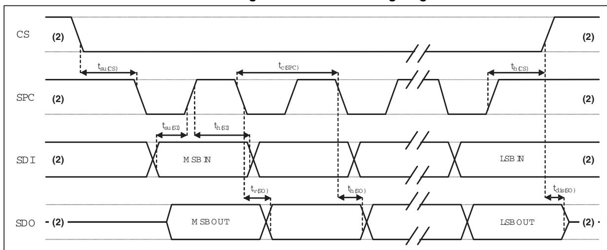
2. Data on CS, SPC, SDI and SDO refer to pins: CS\_A, CS\_G, SCL\_A/G, SDA\_A/G, SDO\_A / SDO\_G.
