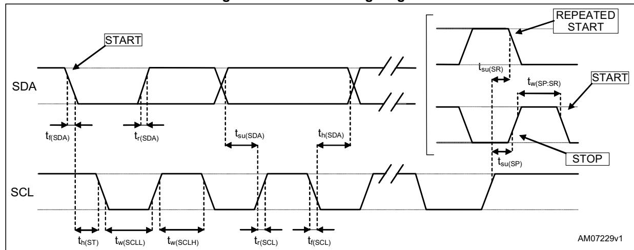
Note: Measurement points are done at 0.2·Vdd\_IO and 0.8·Vdd\_IO, for both ports.
