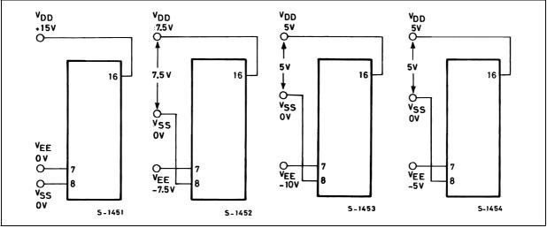
The ADDRESS (digtal-control inputs) and INHIBIT logic levels are : "0"=V<sub>SS</sub> and "1"=V<sub>DD</sub>. The analog signal (through the TG) may swing from V<sub>EE</sub> to V<sub>DD</sub>
