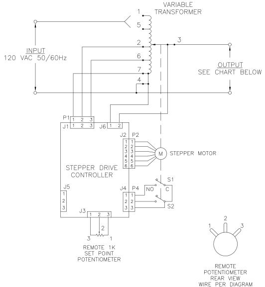
SET POINT ADJUSTMENT: THE OUTPUT SET POINT MAY BE ADJUSTED WITH THE REMOTE 1K POTENTIOMETER PROVIDED OR WITH A 0-5 VDC SIGNAL TO THE J3 CONNECTOR ON THE STEPPER DRIVE CONTROL. MAKE CONNECTIONS TO J3-2(+) & J3-3(-). A NOMINAL +5 VDC SETPOINT SUPPLY IS AVAILABLE AT J3-1 (ADJUSTABLE AT TRIMPOT R22).
