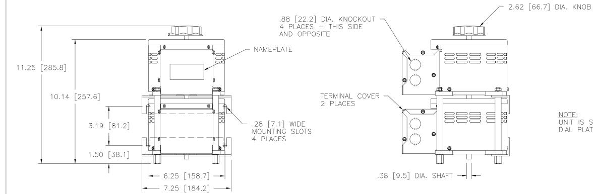
UNIT IS SUPPLIED WITH A 3.75 [95.2] DIA. 0-100 GRADUATED DIAL PLATE FOR PANEL MOUNTING.
