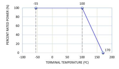
Operating temperature range of -55°C to 170°C. Storage condition: 5°C ~ 35°C, humidity of 40% ~ 75%.
