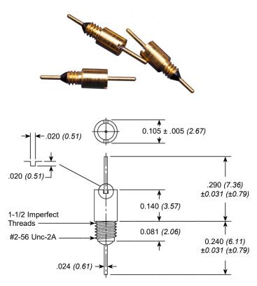
Built and tested in accordance with MIL-PRF-15733. Dimensions in inches *(mm)*
