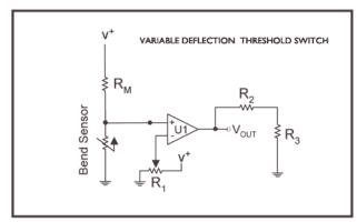
"Resistance to Voltage Converter - use the sensor as the input of a resistance to voltage converter using a dual-sided supply op-amp. A negative reference voltage will give a positive output. Should be used in situations when you want to output at a low degree of bending."
