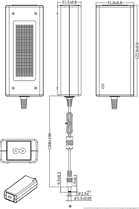
DC Cable: UL1185 16AWG Black 1299 mm + 100 mm Connector:  $2.5 \times 5.5 \times 9.5$  mm, fork type, center "+"
